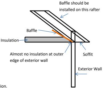
Baffle goes out to top plate, leaving only an inch for insulation.
